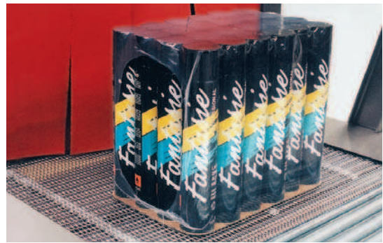
Automatic flat carton insertion to stiffen the packages and improve the palletising.
