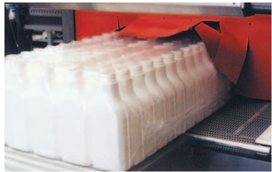
Possibility to get a total package sides closure by film overlapping (even with packages of big dimensions).
